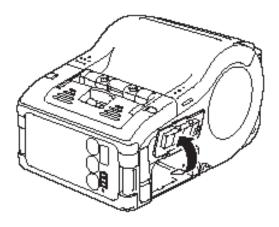
3. Align the battery pack so that its metal terminals (1) are facing the printer and the tab (2) on the battery is up, then insert the battery until it snaps in place.
